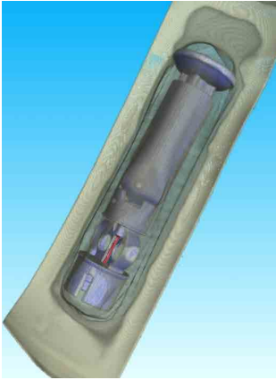
3D CT Scan of Syringe in Bubble Pack
