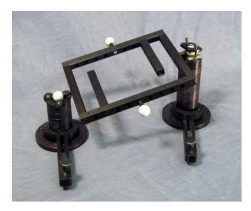
The Universal Fixture provides an easy to use platform for scanning small to mid size parts on most Surveyor Scanning Systems. The fixture consists of a modular fixture frame that can be assembled in various configurations to accommodate many different part sizes. This frame attaches to the two fixture towers, allowing the operator to position the part in virtually any position for scanning.
