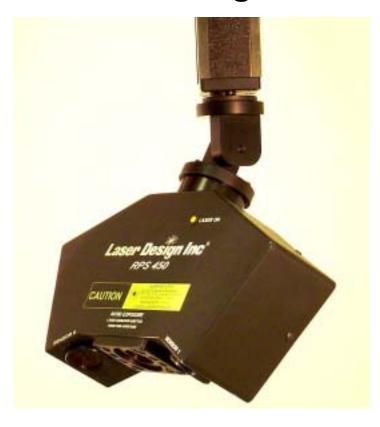
The Laser Mounting Wrist provides the capability to orient the RPS laser probes in numerous orientations to aid in scanning complex geometry. The Laser Mounting Wrist provides a full 360 degrees of rotation around W and 180 degrees of rotation around V with infinite adjustments for both.
