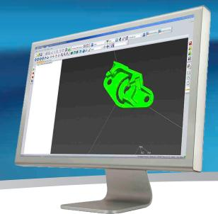
SSC provides optimization for part specularity, data density control, and filtering as well as macro programming capabilities for automating repetitive applications and eliminating operator involvement.
