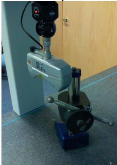
Figure 2: Typical Ball Bar Setup
